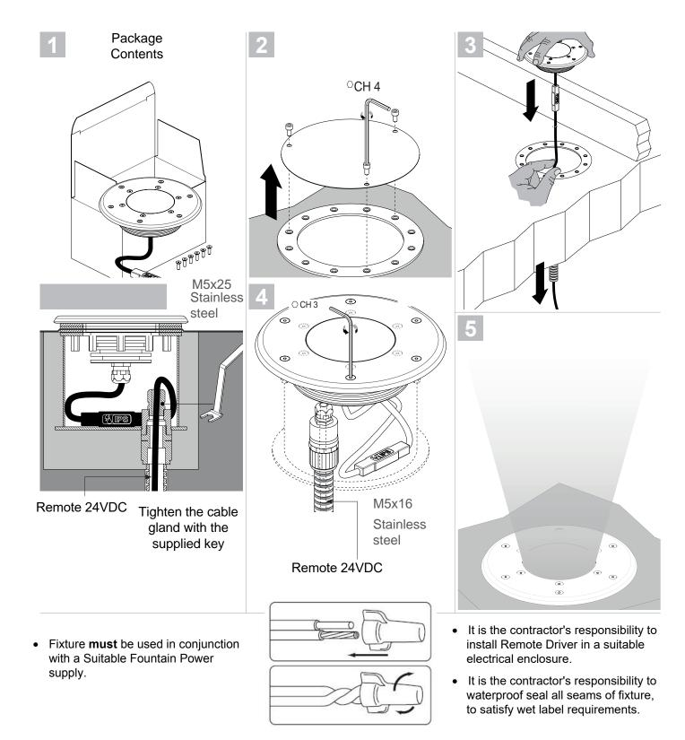
Use gel-filled waterproof wire-nuts for wire connections.
