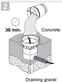
Use 7-12" of drainage gravel - check functionality: fill tube with water and verify full drainage within 30 min. If water remains, please utilize a different drainage system that functions properly. Contractor to seal the conduit with "Great Stuff" aerosol seal.
