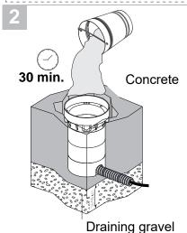
Use 7-12" of drainage gravel - check functionality: fill tube with water and verify full drainage within 30 min. If water remains, please utilize a different drainage system that functions properly. Contractor to seal the conduit with "Great Stuff" aerosol seal.
