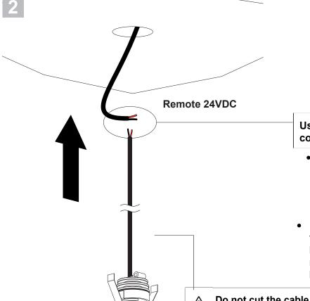
Use wire-nuts for wire connections.
