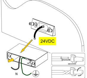
Use wire-nuts for wire connections.
