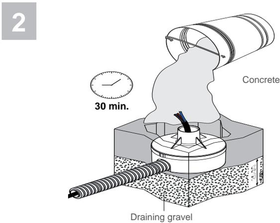
Use 7-12" of drainage gravel - check functionality: fill tube with water and verify full drainage within 30 min. If water remains, please utilize a different drainage system that functions properly. Contractor to seal the conduit with "Great Stuff" aerosol seal that prevents water and moisture penetration for ultimate protection.
