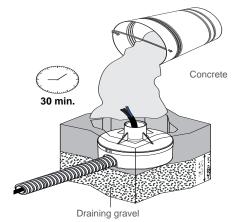
Use 7-12" of drainage gravel - check functionality: fill tube with water and verify full drainage within 30 min. If water remains, please utilize a different drainage system that functions properly. Contractor to seal the conduit with "Great Stuff" aerosol seal that prevents water and moisture penetration for ultimate protection.
