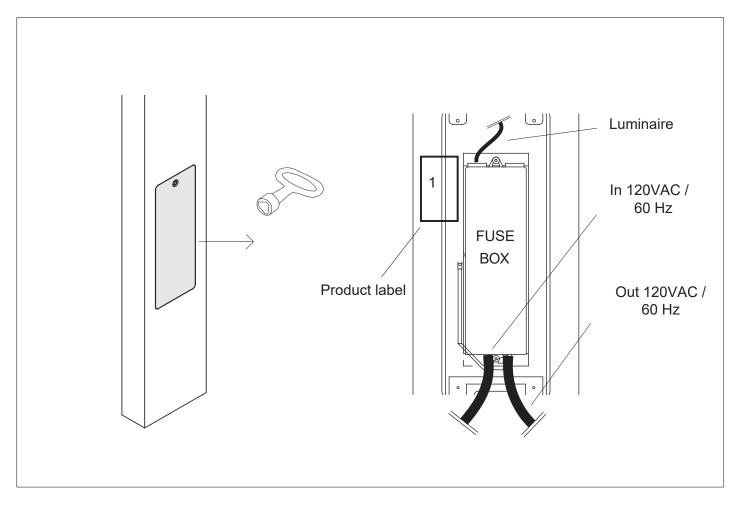
Connect the power supply cable and the lamp cable to the terminal board. It is only necessary to connect the power cord to the Bollard version. The product label is located on the clamping plate of the terminal board. Clamp includes 2x6 A fuses (D01). The fuses are to be tested by an electrician and replaced if necessary.
