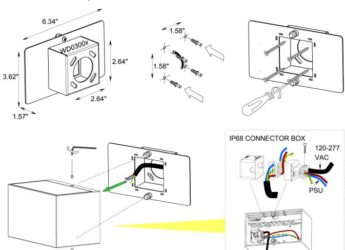
It is the contractor's responsibility to caulk around the edges between the fixture and the mounting surface, to satisfy wet label requirements.
