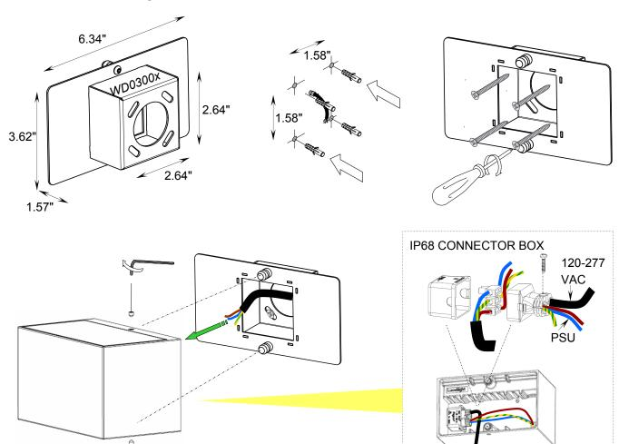
It is the contractor's responsibility to caulk around the edges between the fixture and the mounting surface, to satisfy wet label requirements.
