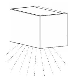
It is the contractor's responsibility to caulk around the edges between the fixture and the mounting surface, to satisfy wet label requirements.
