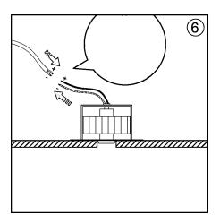
Use wire-nuts for wire connections.
