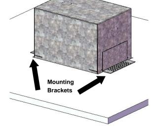
Loosen all four wingnuts slightly and position the housing so that is it recessed in the opening by about ¼".
