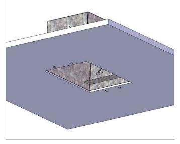
5. Apply fiberglass tape around opening and apply plaster. Sand smooth when dry.
