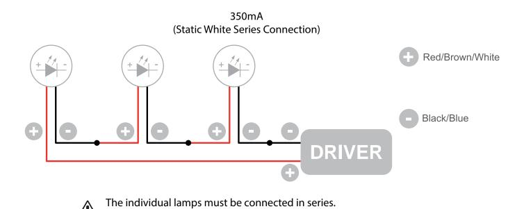
• LED lights work at constant current. When choosing a power supply unit, you need to consider the current
