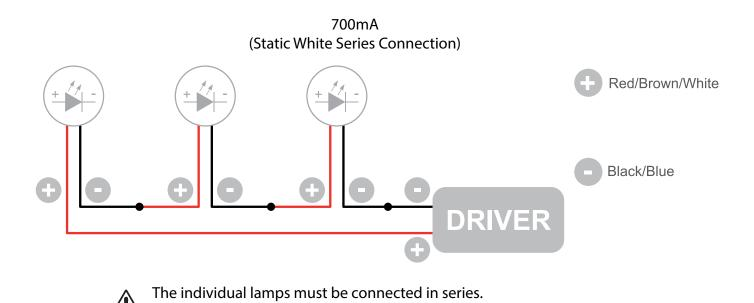
• LED lights work at constant current. When choosing a power supply unit, you need to consider the current! by which the LEDs are driven and their maximum power consumption.
