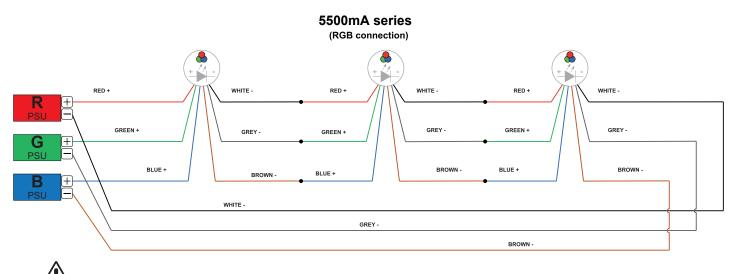
FOR RGB VERSION ONLY: The individual lamps must be connected in series.
