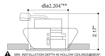
\*\*for metal, wood and plasterboard use standard drill size 2.17" \*\*for concrete use standard drill size 2.205"
