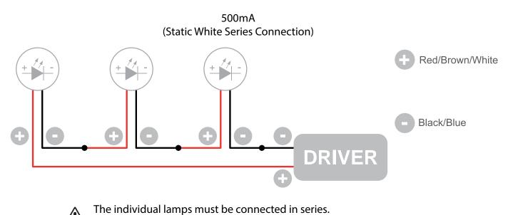
Only power up the system once all the lamps have been connected.
