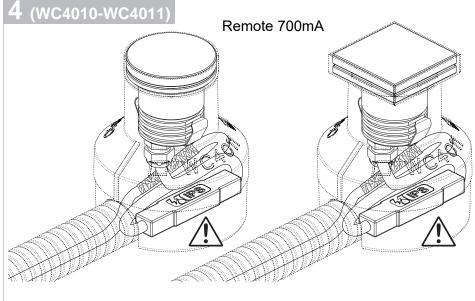
Use conduit Ø0.79" minimum (recommended Ø0.98")
