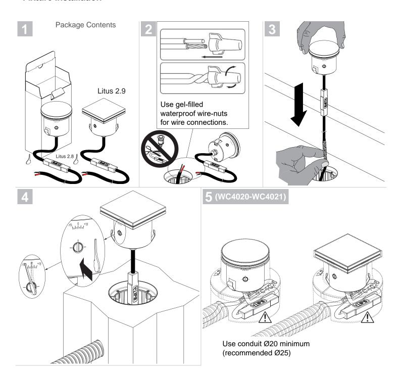
BEAM ADJUSTMENT (fig. 5) When installing adjustable devices, insert the lever provided into the screw to adjust the orientation of the light beam. A screwdriver may also be used.
