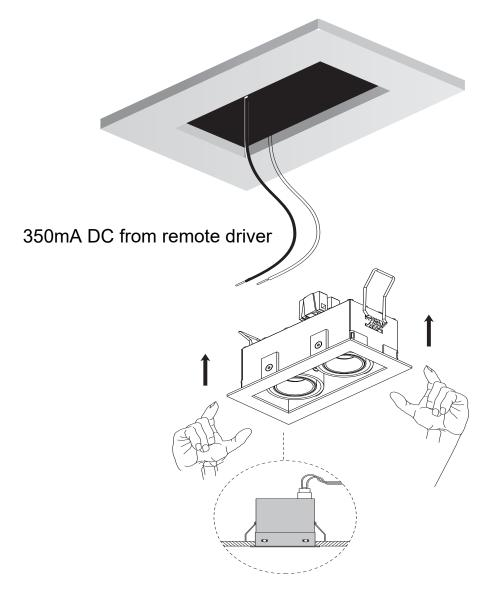
MINIMUM CEILING THICKNESS: 0.039 in MAXIMUM CEILING THICKNESS: 0.984 in
