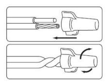
Use gel-filled waterproof wire-nuts for wire connections.
