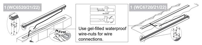
Connect to mains power using a suitable terminal board inside a connection box with the correct ingress protection, in accordance with systems regulations.
