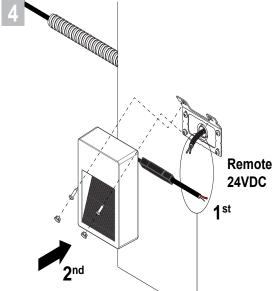
Use gel-filled waterproof wirenuts for wire connections.
