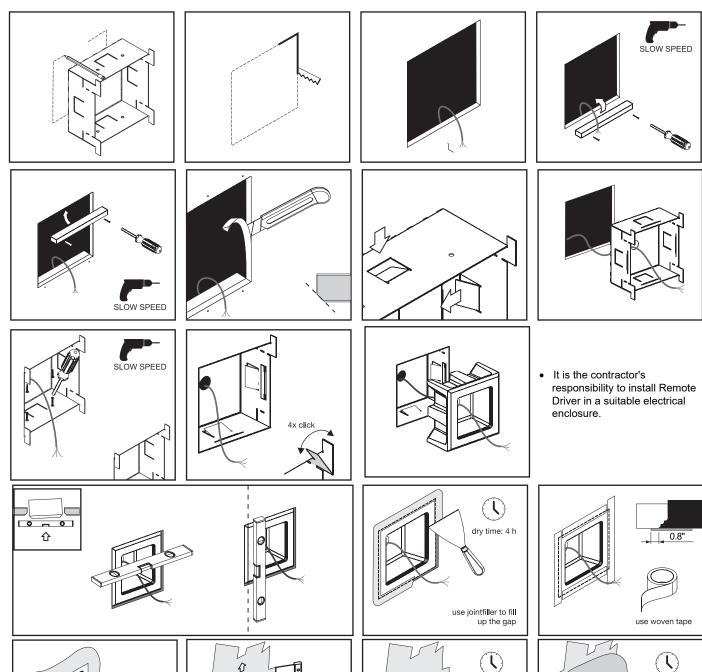
fix the tape with jointfiller
