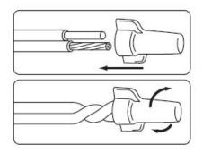
Use gel-filled waterproof wire-nuts for wire connections.
