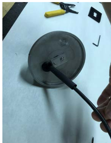
Fixture cord after modification
