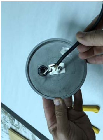
Fixture cord before modification
