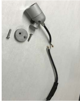
Fixture cord after modification
