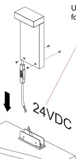
Use gel-filled waterproof wire-nuts for wire connections.
