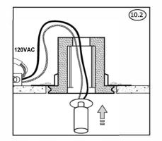
• Use wire-nuts for wire connections.
