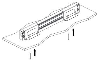
Concealed recessed spotlights: carefully apply plaster and smooth over the casing and screw holes. Carefully clean the inside of the casing. All plaster residue must be removed.
