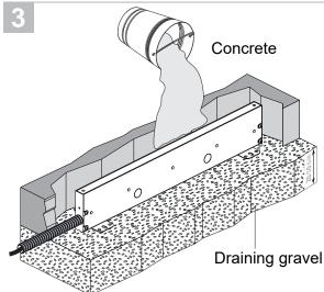
Use 7-12" of drainage gravel - check functionality: fill tube with water and verify full drainage within 30 min. If water remains, please utilize a different drainage system that functions properly. Contractor to seal the conduit with "Great Stuff" aerosol seal that prevents water and moisture penetration for ultimate protection.
