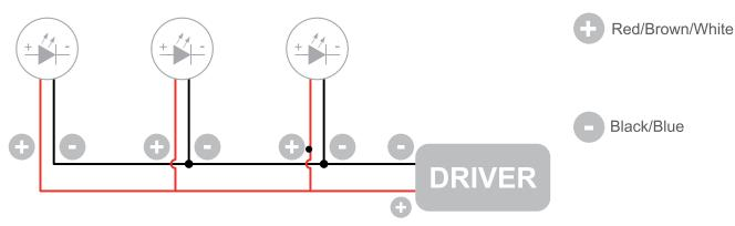
The individual lamps must be connected in parallel. Only power up the system once all the lamps have being connected.
