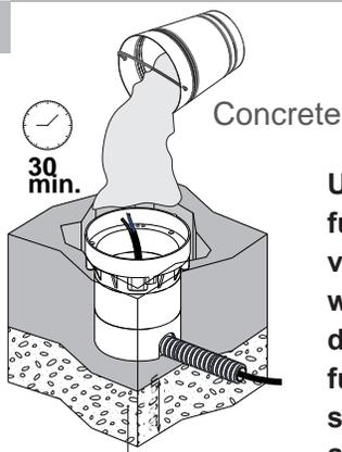
Use 7-12" of drainage gravel - check functionality: fill tube with water and verify full drainage within 30 min. If water remains, please utilize a different drainage system that functions properly. Contractor to seal the conduit with "Great Stuff" aerosol seal that prevents water and moisture penetration for ultimate protection.
