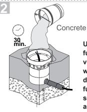
Use 7-12" of drainage gravel - check functionality: fill tube with water and verify full drainage within 30 min. If water remains, please utilize a different drainage system that functions properly. Contractor to seal the conduit with "Great Stuff" aerosol seal that prevents water and moisture penetration for ultimate protection.
