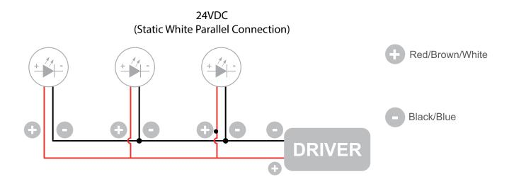
The individual lamps must be connected in parallel. Only power up the system once all the lamps have being connected.
