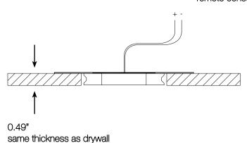
Slice is without mounting formwork and can be installed in a layer of drywall just 0.49" thick. Because it can be inspected from the front it does not need any inspection hatch.
