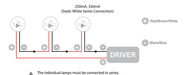
Only power up the system once all the lamps have been connected.
