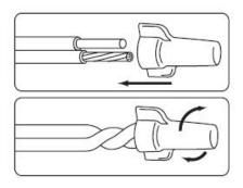
Use gel-filled waterproof wire-nuts for wire connections.
