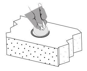
Its successful function can be guaranteed only upon immediate use after installation of the fittings. Long term installation of the spots is subject to dust and dirt infiltration between the glass frame of the fitting and edges of the box, which works as a binding element. In this case the use of the suction cup would not be efficient enough to perform the removal.
