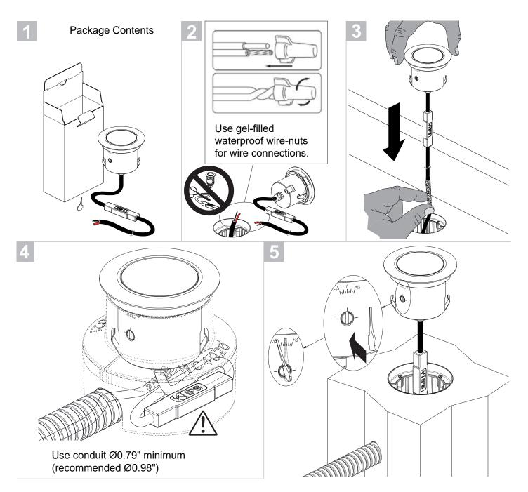
BEAM ADJUSTMENT (fig. 5) When installing adjustable devices, insert the lever provided into the screw to adjust the orientation of the light beam. A screwdriver may also be used. When you reach the limit stop (±15°), do not force it with the lever as this could compromise the device's ingress protection and its functioning.
