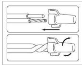
Use gel-filled waterproof wire-nuts for wire connections.
