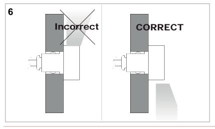
It is the contractor's responsibility to caulk around the edges in between the fixture and the mounting surface, to satisfy wet label requirements.
