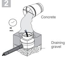
Use 7-12" of drainage gravel - check functionality: fill tube with water and verify full drainage within 30 min. If water remains, please utilize a different drainage system that functions properly. Contractor to seal the conduit with "Great Stuff" aerosol seal that prevents water and moisture penetration for ultimate protection.
