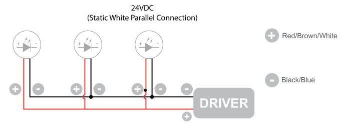
The individual lamps must be connected in parallel. Only power up the system once all the lamps have being connected.
