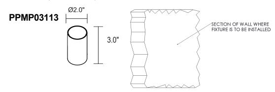
Drill pilot hole for core drilled housing through wall
