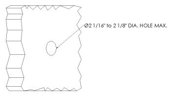
Apply epoxy to sides of newly drilled opening, insert core drilled housing into pilot hole and make level
