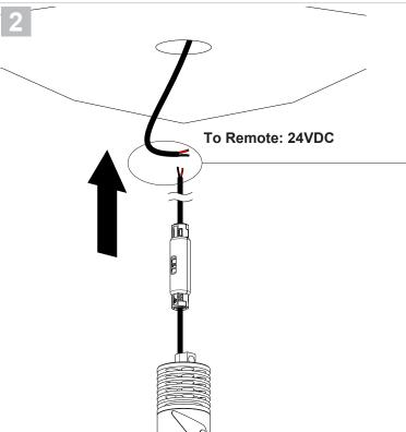
• Use gel-filled waterproof wire-nuts for wire
