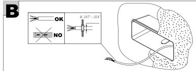
It is the contractor's responsibility to install Remote Driver in a suitable electrical enclosure.
