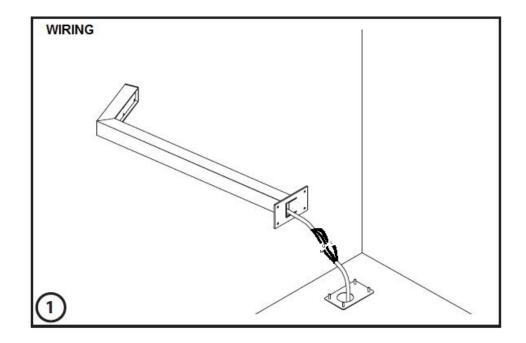
Always Use gel-filled waterproof wire nuts to connect wires.
