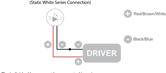
The individual lamps must be connected in series. Only power up the system once all the lamps have been connected.
