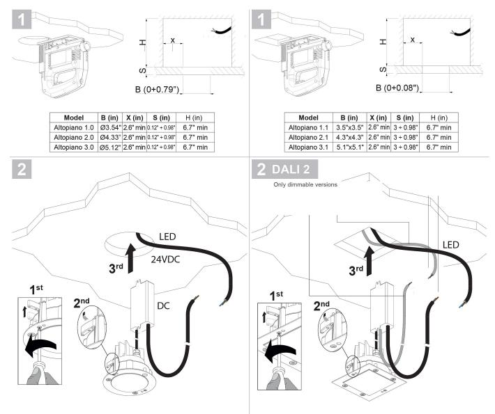
Use a terminal block conforming to EN 60998-2-1 or EN 60998-2-2 with a 3-terminal type, with a nominal voltage of 400V, with a connection capacity of 1.00 to 2.00 mm<sup>2</sup>.
