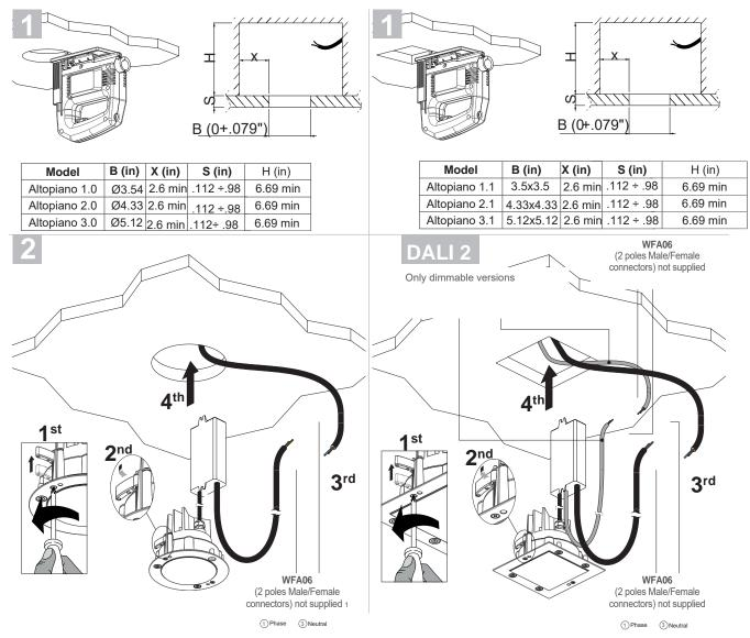
Use a terminal block conforming to EN 60998-2-1 or EN 60998-2-2 with a 3-terminal type, with a nominal voltage of 400V, with a connection capacity of 1.00 to 2.00 mm<sup>2</sup>.
