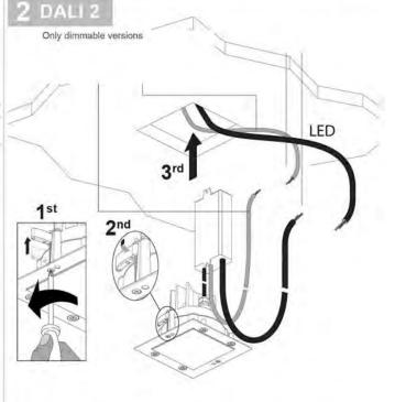
Use a terminal block conforming to EN 60998-2-1 or EN 60998-2-2 with a 3-terminal type, with a nominal voltage of 400V, with a connection capacity of 1.00 to 2.00 mm².
