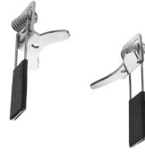
WGA02 Retaining Spring Clip Use for ceilings 3/64" min. to 1 3/8" max. thick
