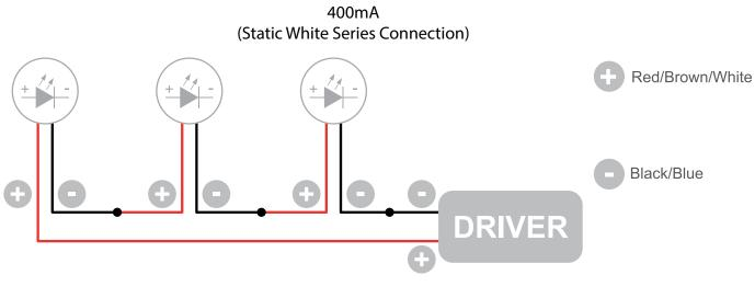
The individual lamps must be connected in series. Only power up the system once all the lamps have been connected.
