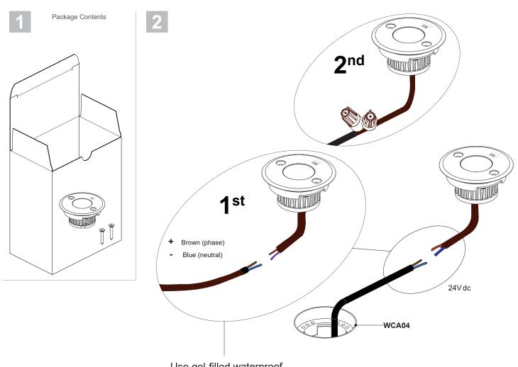
Use gel-filled waterproof wire-nuts for wire connections.
