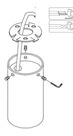
Use gel-filled waterproof wirenuts for wire connections.
